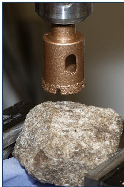
Fig. 2: Diamond hole saw, together with forest marble rock, held in the jaws of a milling vice. Note the shell on the top surface of the specimen directly under the cutter.
