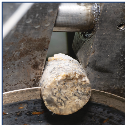
Fig. 5: Core held in the vice of the precision saw while being cut. The V-groove can just be seen behind the sample, on the right.
