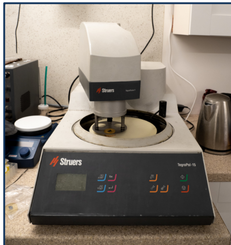
Fig. 3: Struers Polisher, fitted with an abrasive disc. Various programmes are available for grinding and polishing, with or without water lubrication.
